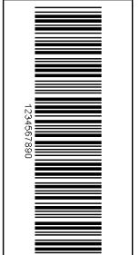
Case 3 : Gap paper ( Label: 50(H) \* 100(W) \* gap 3 ) ^Q50,0,0 ^W100. Rotate 90°, it becomes ^Q100,0,0 ^W50 + ^XSET,ACROSS,1 ( cross label command ). It will print out below labels with 100mm (H) \* 50mm (W).
